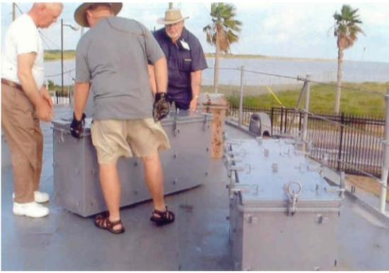
Ready to move! **Robin's** 20mm boxes ready to be placed in their positions. As can be seen in this view, the shrapnel shields are missing on the boxes and will have to be fabricated.
